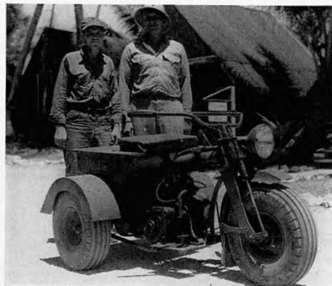
A motor driven cycle was built with "Jap" materials.
