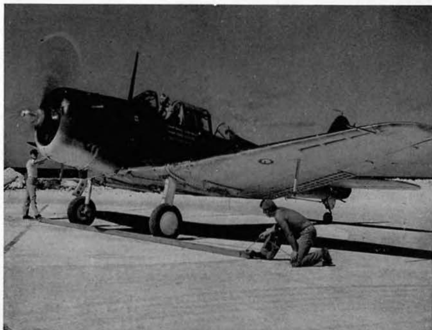
The first plane rolls on the "Rose" and his compass is checked.
